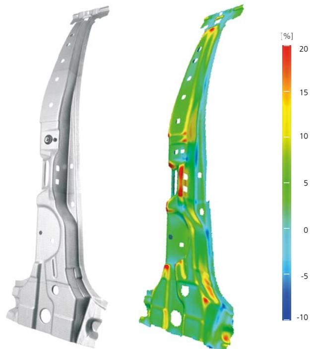
The optical forming analysis using ARGUS has become a proven tool for evaluating forming processes and verifying simulations. In particular, the precise, accurate and user-independent measuring procedure as well as the surface representation of deformation distributions strengthened the acceptance of this measuring technology. This unique possibility to measure complex sheet metal parts with a high scanning density opens up new aspects for the verification of forming simulations.
